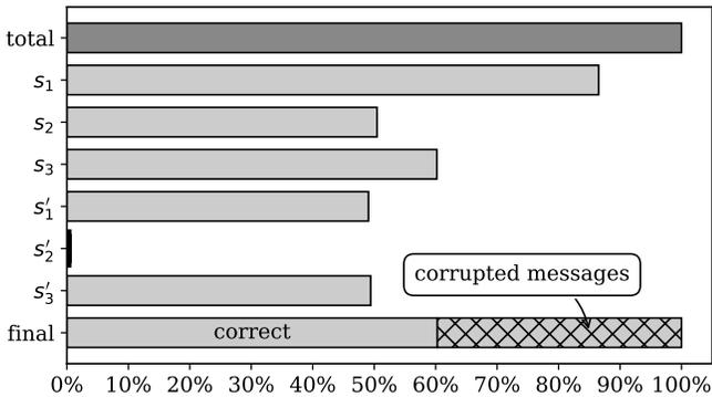
Fig. 6. Error identification statistics, based on Comm-B replies received at TU Delft from 12:00 to 13:00 UTC, September 7, 2017
