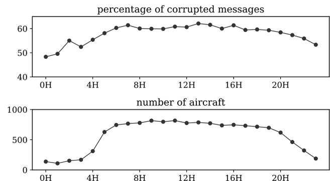
Fig. 10. Percentage of corrupted ADS-B messages and number of aircraft per hour on May 30, 2018, in Delft, the Netherlands
