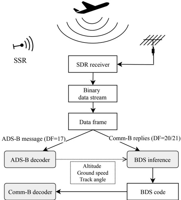
Fig. 1. The Mode-S inference and decoding pipeline
