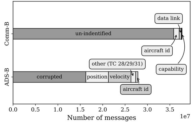
Fig. 3. Number of ADS-B message and Mode-S Comm-B replies received in 24 hours, May 30, 2018
